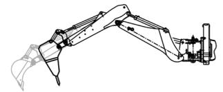
Hydraulikhammer inst. + Teleskoparm
